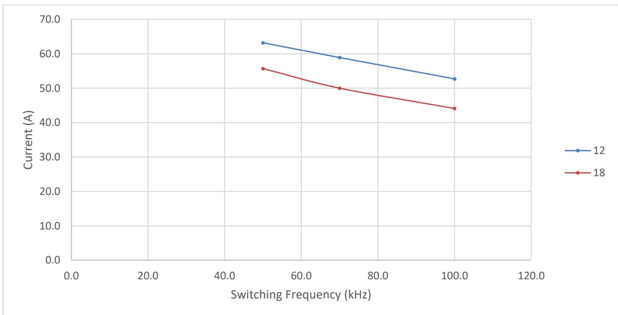
Inverter Continuous Safe Operating Area for Selected Switching Frequencies in kHz
