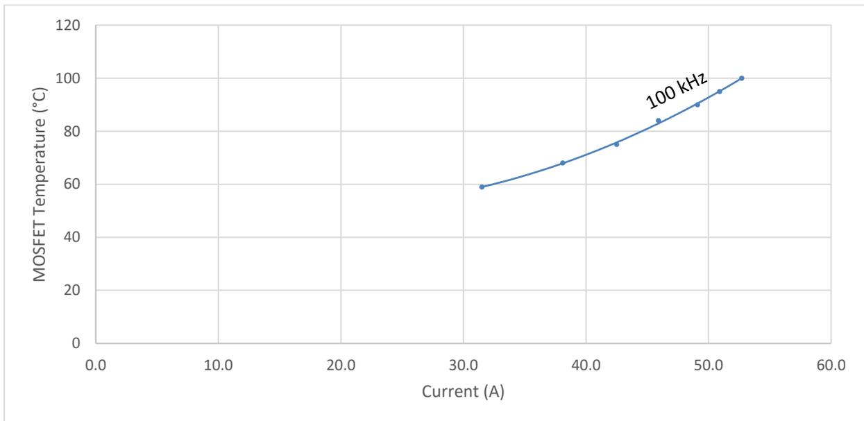
MOSFET Package Temperature for Selected Switching Frequencies in kHz
