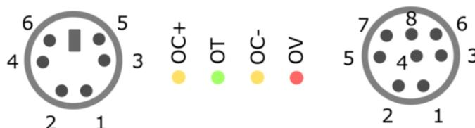
The SPI-DCI-35V-50A-NI-NF-1 features standard, shielded miniDIN connectors, and polarized male headers in parallel, to control and monitor the power switches. Additionally, a male header connected to the cable shield is provided as well as headers for the supply input. The H-bridge connections are made using threaded M4 studs, preferably through spade or ring terminals.
