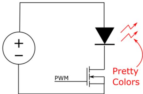
Figure 3: An Ideal Buck Converter (But a Bad Circuit Idea)
