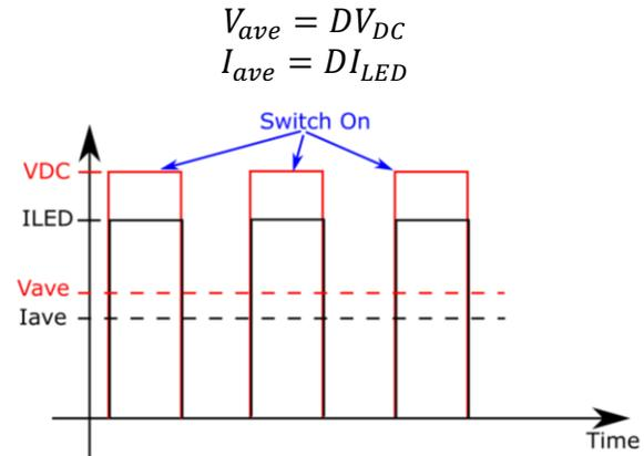
Figure 4: Ideal Buck Converter Waveforms
